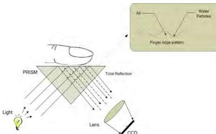
Fig 1. Optical fingerprint sensing by frustrated total internal reflection
